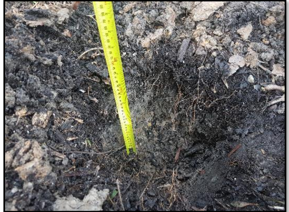
Photo 2: Image of TP01 with brown silty sand observed above grey sandy clay with red and orange mottling. Representative of sample TP01 0.2-0.3.
