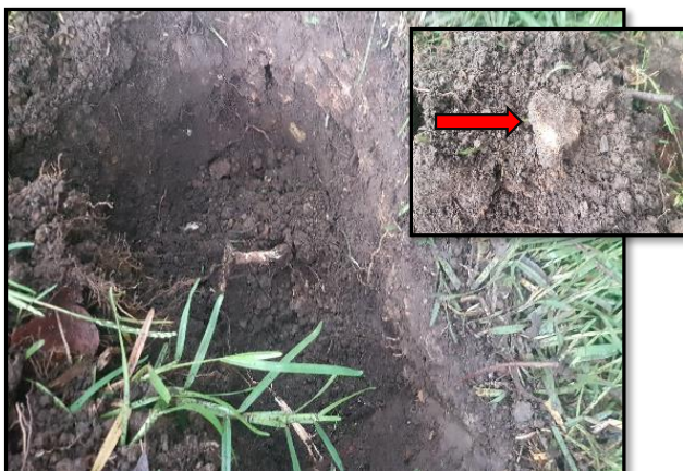
Photo 11: Image of TP03 located at 9 Fig Tree Street, with (insert) sandstone blocks observed within brown silty sand fill layer.
